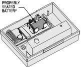
Figure 7. Battery Insertion
